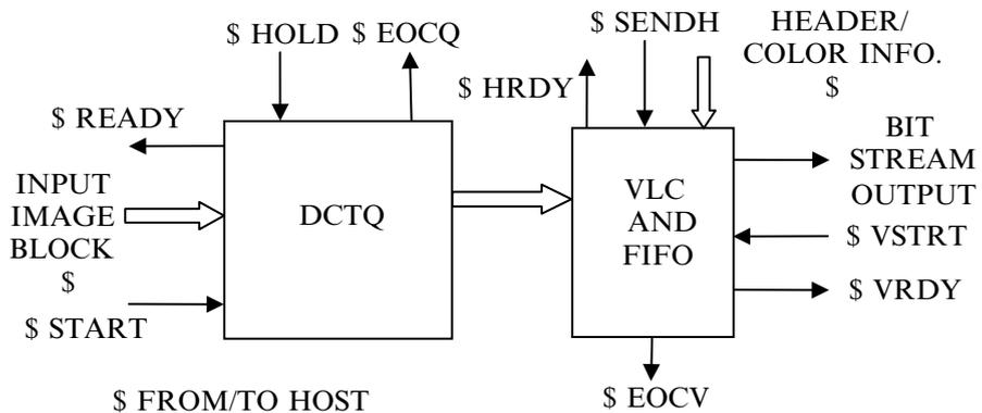
**Fig. 15.8 Basic architecture of the implemented MPEG 2 encoder**
