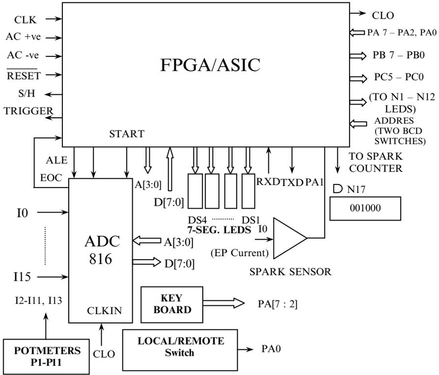
**Fig. 15.4 FPGA board of the electrostatic precipitator controller**
