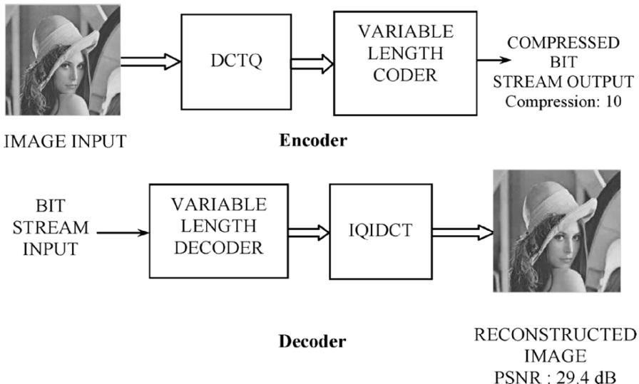
**Fig. 15.5 Basic architecture of JPEG/ H.261/H.263/MPEG codec**
