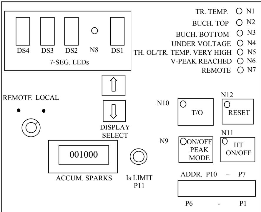
Fig. 15.1 Front panel of electrostatic precipitator controller
