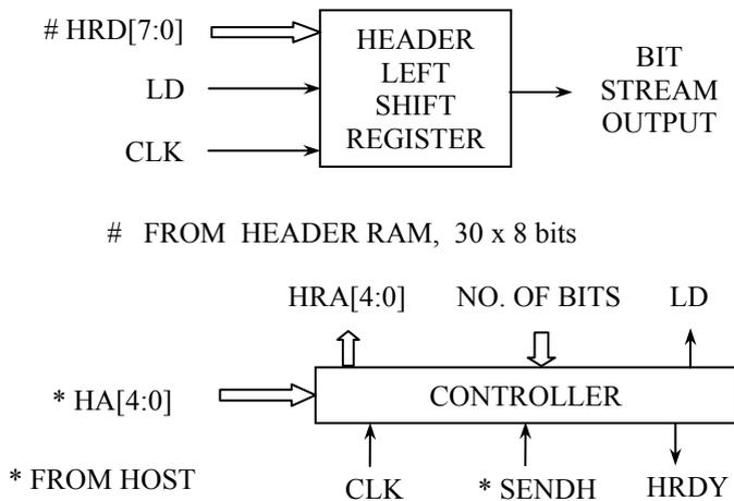
**Fig. 15.11 Header serial output converter**
