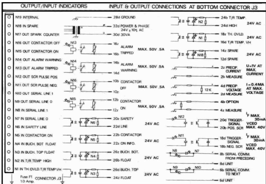
Fig. 15.2 Rear panel of electrostatic precipitator controller
